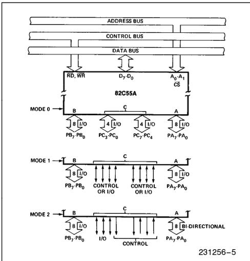
Figure 5. Basic Mode Definitions and Bus Interface
