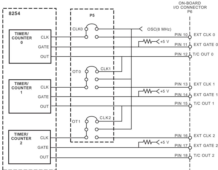
Fig. 1-6 — 8254 Timer/Counter Circuit Block Diagram
