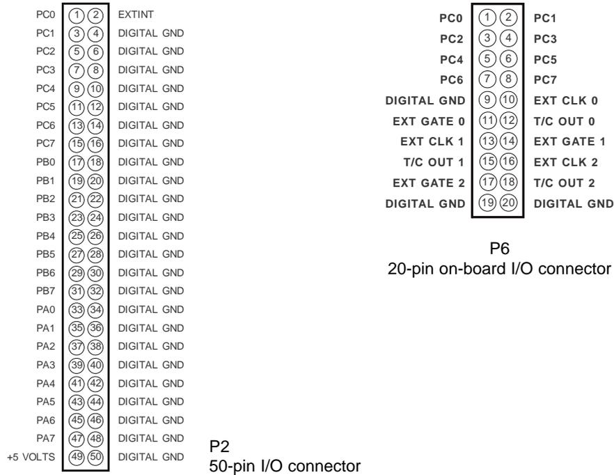
Fig. 2-1 — P2 and P6 I/O Connector Pin Assignments
