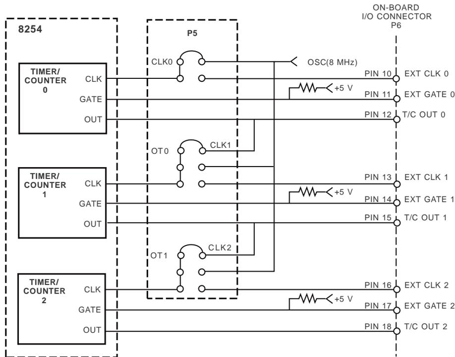
Fig. 4-1 — 8254 Timer/Counter Circuit Block Diagram
