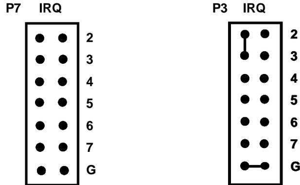
Fig. 1-2 — Interrupt and Interrupt Channel Jumper, P3 and P7
