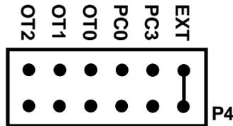
Fig. 1-4 — Interrupt Source Select Jumper, P4
