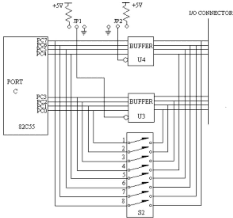
Fig. 1-8 — Port C Buffer Circuitry
