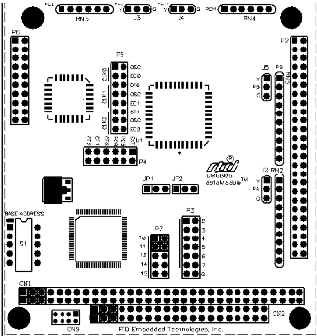
Fig. 1-1 — Board Layout Showing Factory-Configured Settings
