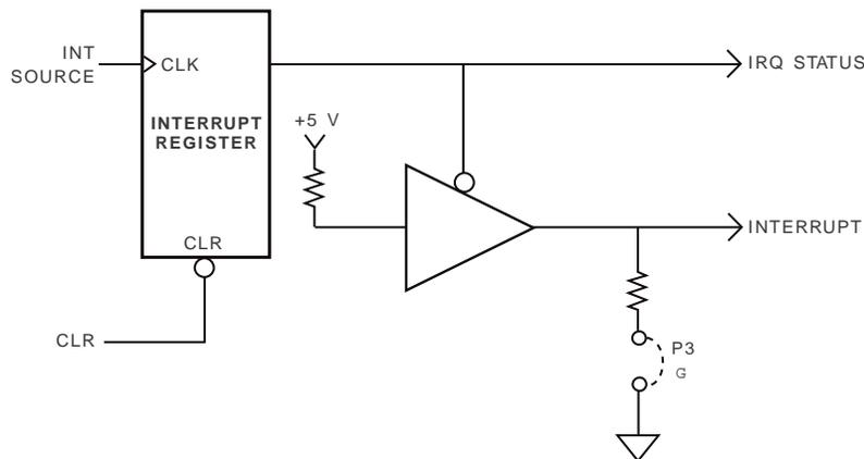
Fig. 1-3 — Pulling Down the Interrupt Request Line
