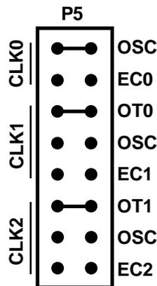
Fig. 1-5 — 8254 Timer/Counter Clock Source Jumpers, P5
